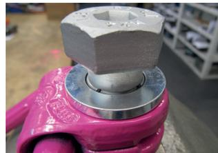
Pic. 9: Retaining ring positioned as circumferential in the recess
