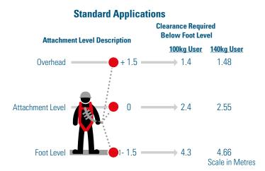
The DSL has been independently tested in all the worst case scenerios. In all cases impact forces remain below 6kN even when attached below at maximum extension or with both legs attached below at maximum extensions. SpanSet DSL tested to be fit for purpose.
