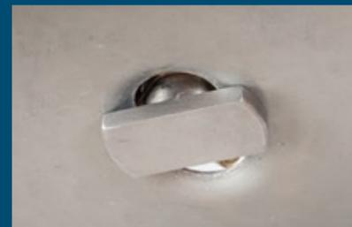
The base clamp, which is firmly connected to the ratchet, rests on the entire surface and ensures optimum force distribution. Even under high loads, deformation of the perforated plate is avoided.
