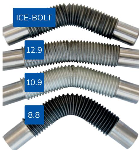
The thread of the ICE-Bolt proves itself in the prism bending test. The test shows: the ICE-Bolt masters static and dynamic WLL safely.
